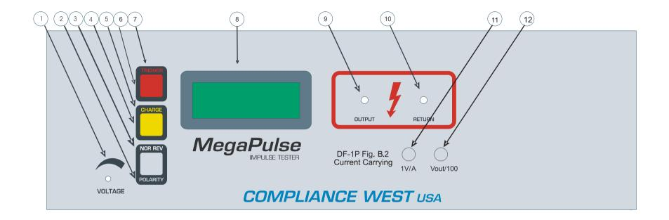
Figure 1. Controls, Indicators, Connectors – MegaPulse DF-1P Fig B.2 Current Carrying Front Panel
