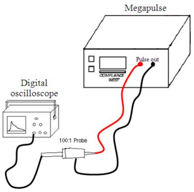
Figure 3: Waveform Measurement Setup
