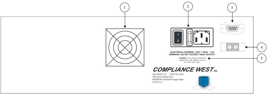
Figure 2. Controls, Indicators, Connectors – MegaPulse DF-1P Fig B.2 Current Carrying Rear Panel
